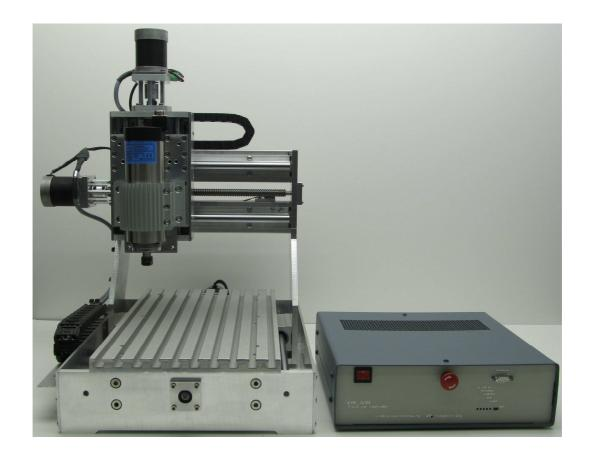
Desktop-miniCNC-Portal-Maschine for CNC-Education and Training with 4-Axis-CNC-Controller und PC-Controlsoftware. The CNC-control works with CAM-files in G-Code according to DIN 66025.
